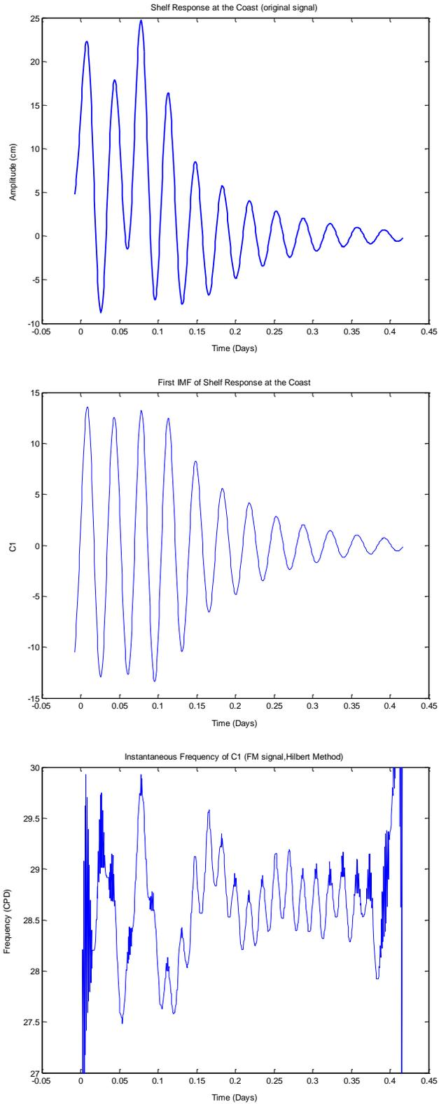
Figure 2. Coastal Shelf Response generated by a KdV soliton train (Top). C1, first IMF obtained by EMD analysis of the Shelf Response (Middle) and C1's Instantaneous Freq. by the Hilbert Method (Bottom).
