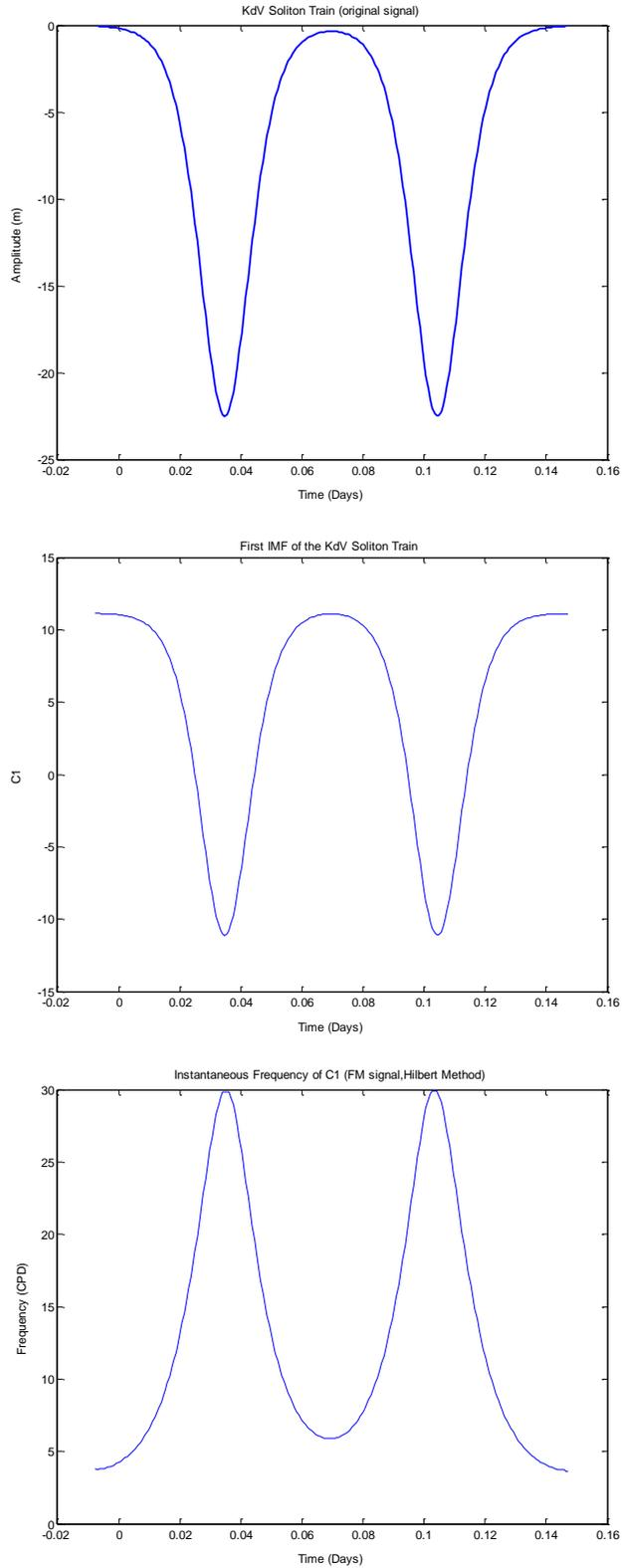
Figure 1. Original offshore KdV soliton train, peaks separated by 100 minutes (Top). First IMF (C1) obtained by EMD analysis (Middle) and C1's Instantaneous Frequency (Bottom).
