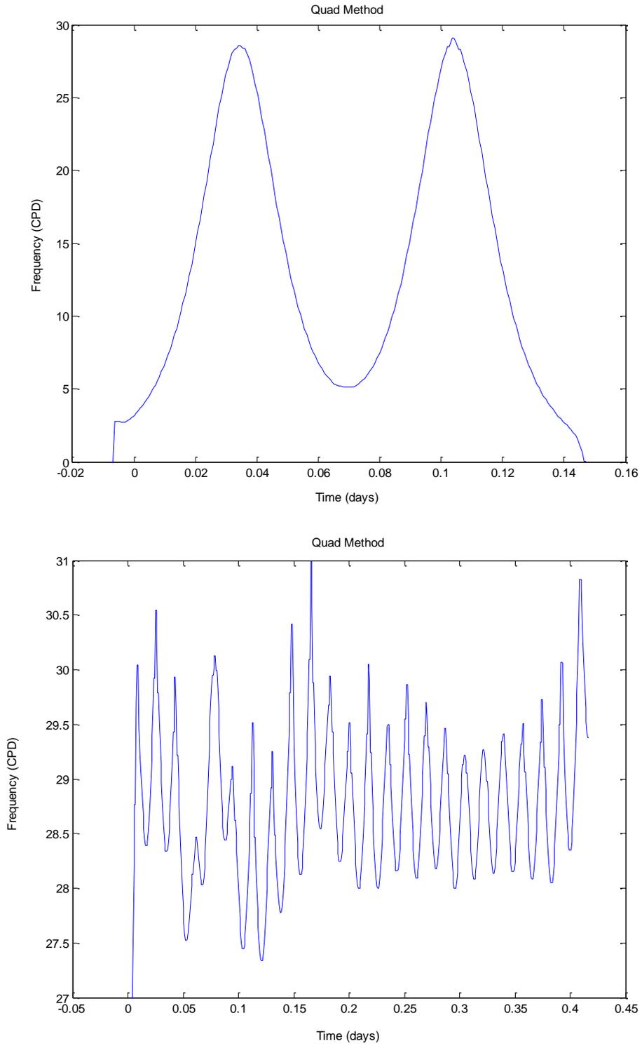
Figure 3. KdV Soliton Train's Instantaneous Frequency (Top). Shelf Response's Instantaneous Frequency (Bottom). Both Instantaneous Frequencies were obtained by the Quad Method.
